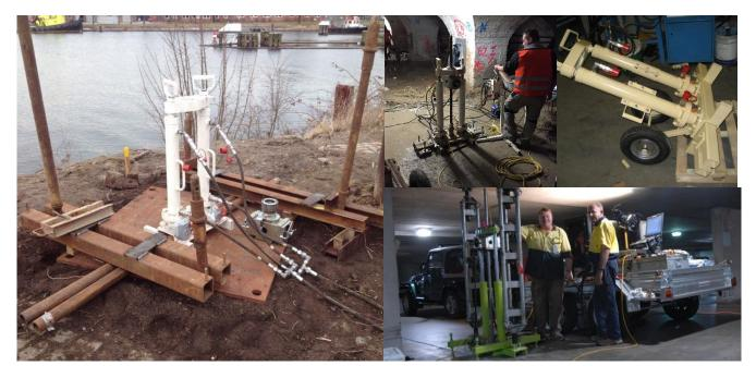
The Geomil Equipment Fox-150 stand-alone CPT system is a versatile unit designed to be used in a wide range of applications. Detachable mounting supports allow the system to be placed on any base.
