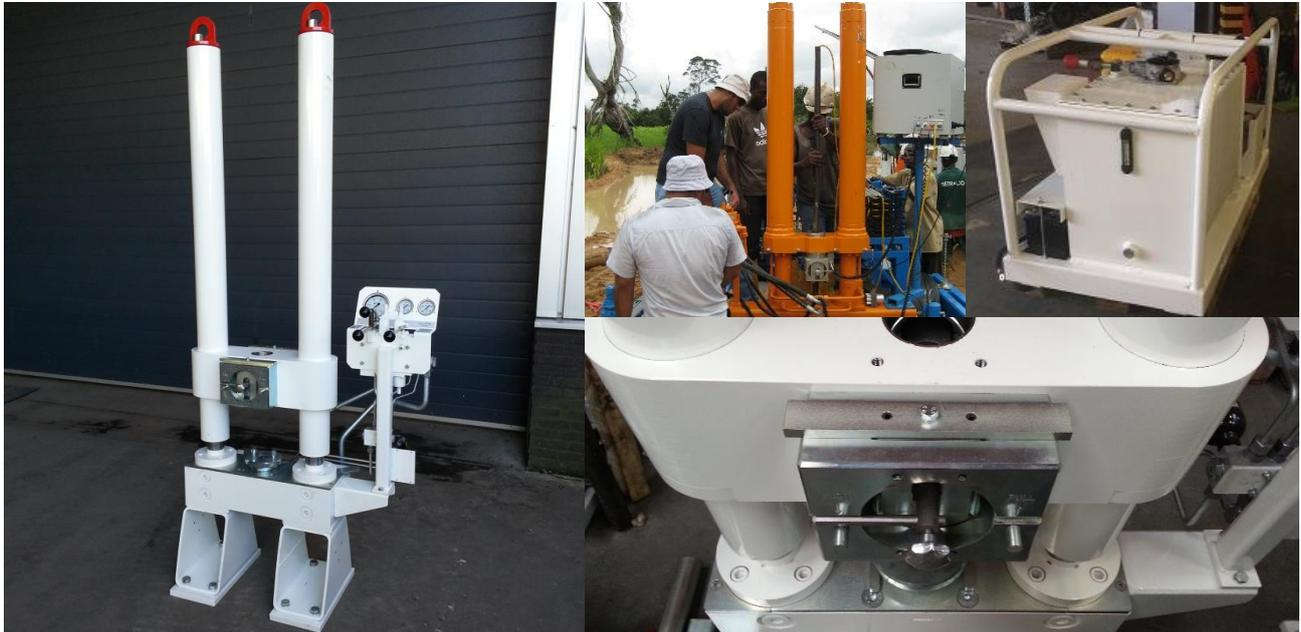
The Geomil Equipment Fox-200 stand-alone CPT system is a versatile unit designed to be used in a wide range of applications. Detachable mounting supports allow the system to be placed on any base, varying from a steel skid to a truck platform, or an excavator to a jack-up platform or barge.
