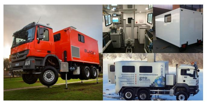
Geomil Equipment's Grizzly is the universal concept for a fully ballasted truck for Cone Penetration Testing (CPT). Its design brings unmatched advantages over conventional systems. The complete CPT installation (load bearing sub-chassis construction, hydraulic system, controls, working cabin and respective interior) comes as a separate unit and can be mounted on nearly any heavy duty, three axle truck, regardless of truck brand.
