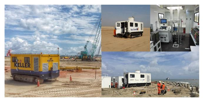
Geomil Equipment Panther series are fully ballasted and completely enclosed, track mounted Cone Penetration Testing (CPT) system.
